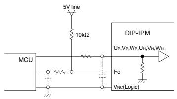
Note: The setting of RC coupling at each input (parts shown dotted) depends on the PWM control scheme and the wiring impedance of the printed circuit board.
